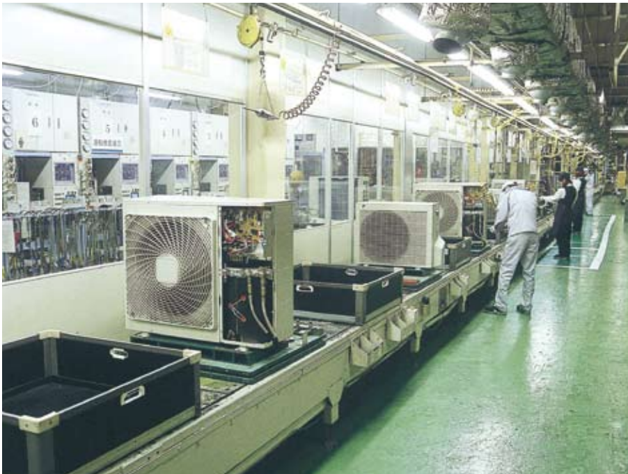
Daikin assembly line for outdoor air-conditioning units (photo courtesy of Daikin Shiga Plant)
