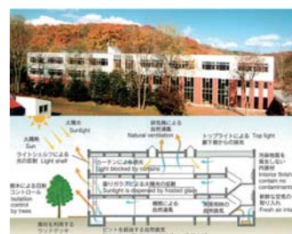
The simple building form, exterior insulation and highly-insulative sash windows
