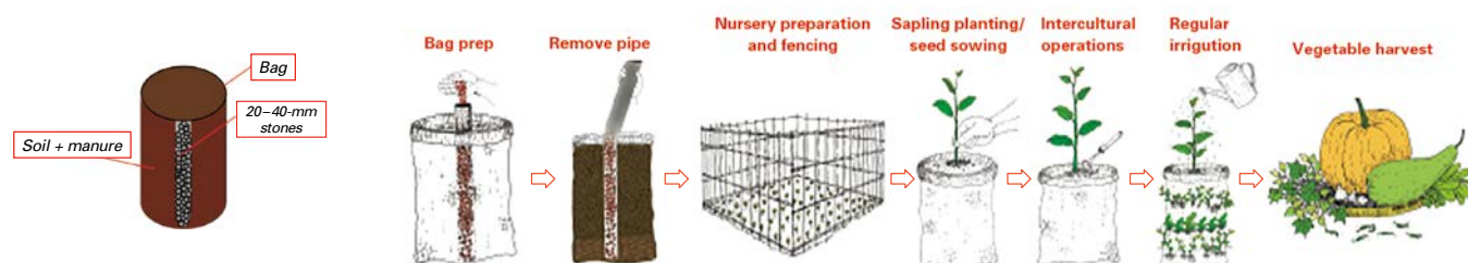
Figure 1. Steps in setting up a sack garden.
